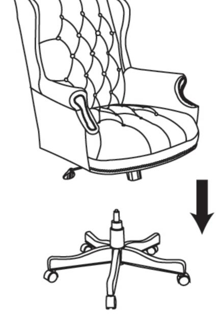
Insert and loosely tightened all screws. When assembly is completed, fully tighten all screws before using. This chair is only intended for sitting, any other use will void the warranty.
